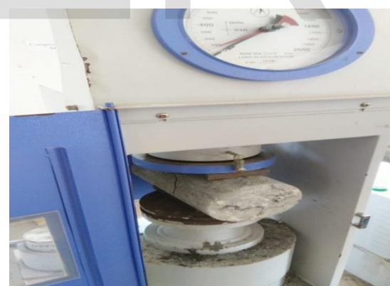
Figure 3. Split tensile test
