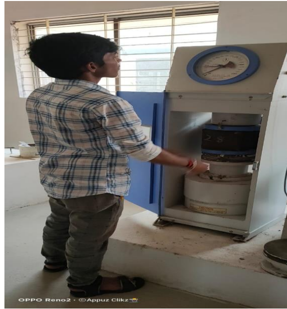
Figure 2. Compressive test on concrete Table 1. Compression Test Results
